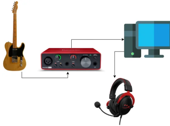
Figure 10. DAW, Interface, and PC Connection
